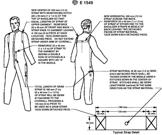
FIG. 7 Details of Safety Grab Straps
